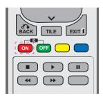
2 If you press the left/right buttons or press the ON button repeatedly, the Picture ID cycles through OFF and 1 to 4.Assign the ID you want.
